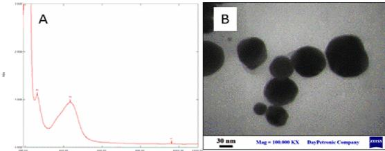
Fig. 2:A:Cr-AgNPs plasmon peak at 434.50 nm.; B: TEM image of Cr-AgNPs with the average size of 30 nm.
